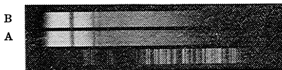
Fig. 3.—The absorption spectra of neodymium chloride (A) and nitrate (B) dissolved in methyl alcohol. (0.0119 mol., 10 cm.)
