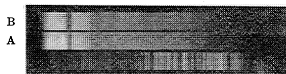
Fig. 5.—The absorption spectra of neodymium chloride (A) and nitrate (B) dissolved in acetone. (0.0119 mol., 10 cm.)
